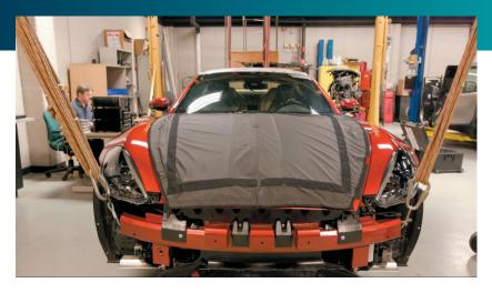
Like many OEMs, Karma realizes that simulation cannot replace physical testing entirely, but Karma staff are convinced that it helps them to achieve better NVH performance in less time. A proper combination of test and simulation allows engineers to determine whether a simulation model represents the reality as closely as possible. But it also yields more detailed insights, such as how to include damping in the model, or how to deal with so-called hybrid approaches.
