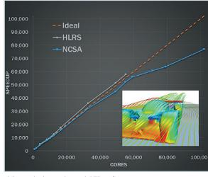
This graph shows the scalability of STAR-CCM+ on National Center for Supercomputing Applications (NCSA) and High Performance Computing Center Stuttgart (HLRS) supercomputers.
