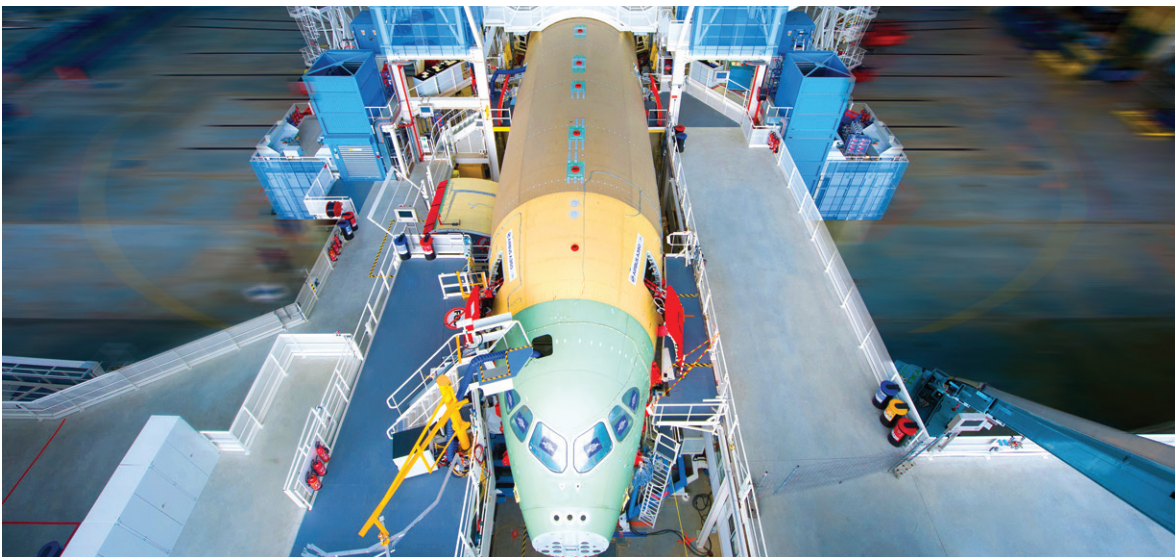
Major components and sections of the A350 XWB are manufactured at Airbus facilities in Germany, Spain, France and the United Kingdom, then shipped to the final assembly line in Toulouse, France. Photo Credit: AIRBUS S.A.S.2012 Photo by e'm company / H.GOUSSÉ.
