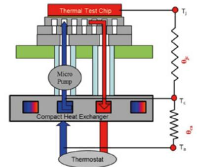
Figure 18. Schematic of the system thermal resistance analysis.
