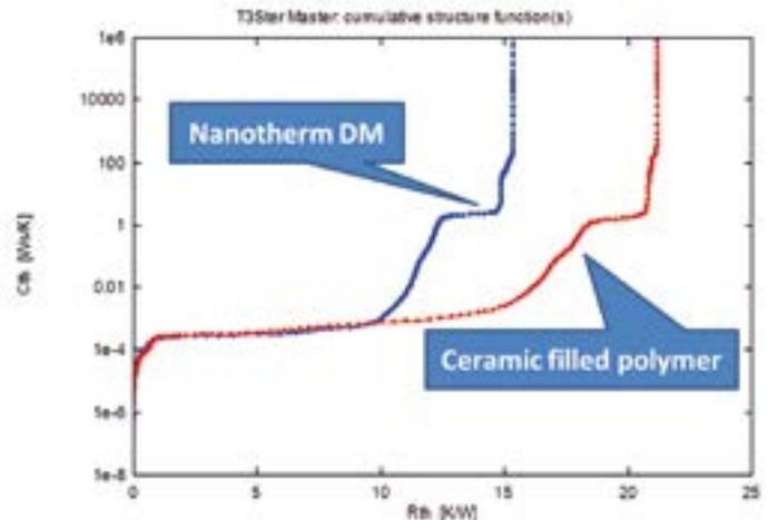
Figure 9. Structure functions of Nanotherm DM
