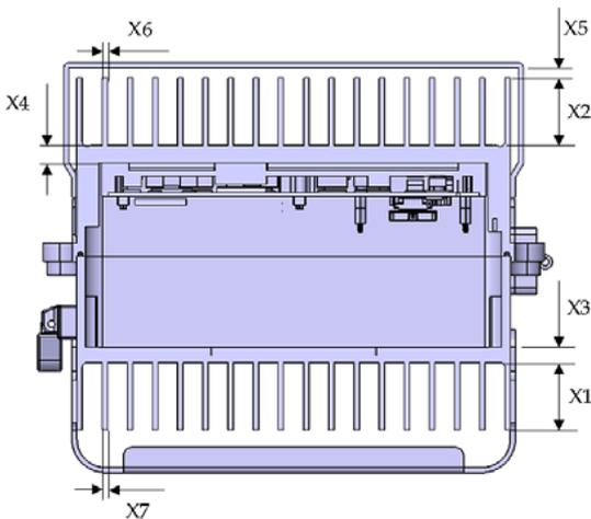
Figure 2. Typical radio access station heat sink variables
