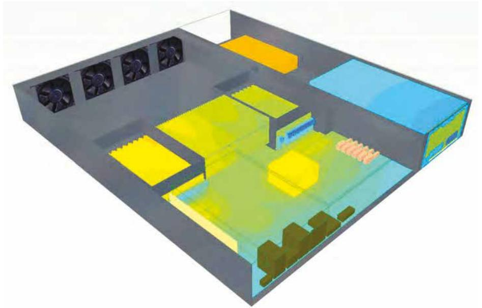
**Figure 1.** FloTHERM isometric view of thermal design shows chassis, motherboard (with dual processors and memory slots side-by-side), fans, and the hard-disk drive (HDD) behind the PSU. The temperature range here assumes an inlet temperature of 27°C. The air duct on top is elided for visualization purposes.
