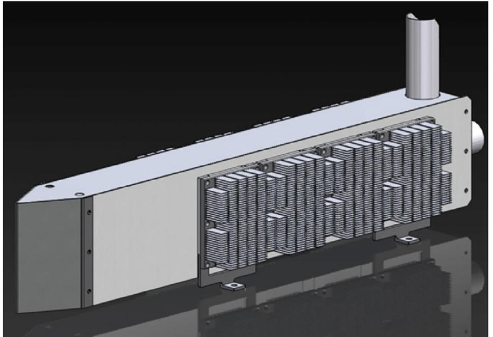
**Figure 2.** The positions of the external heat exchangers that resulted in the highest average power generation for the system
