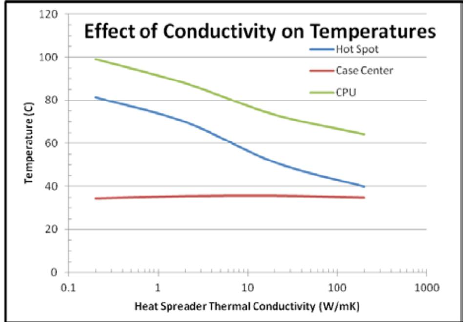
Figure 6. Effect of thermal conductivity of the case on temperatures
