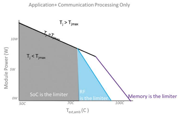
Figure 3. Thermal Cooling Capability Envelope for AP+CP work load.
