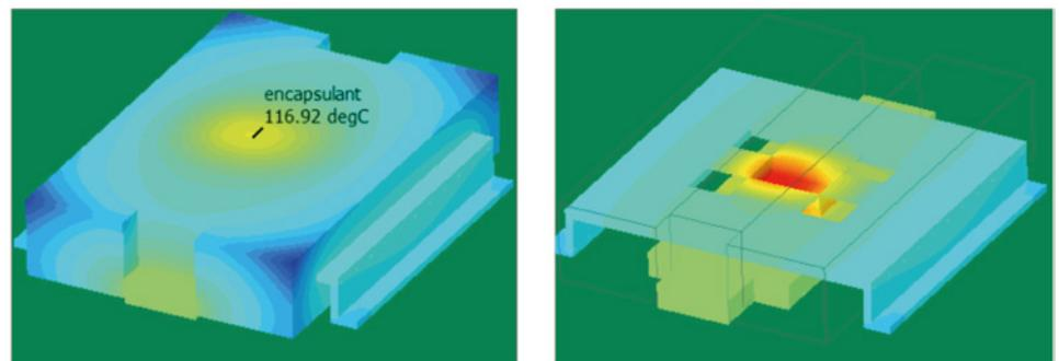
Figure 3. Temperature plots for the package in still air at 85 °C.
