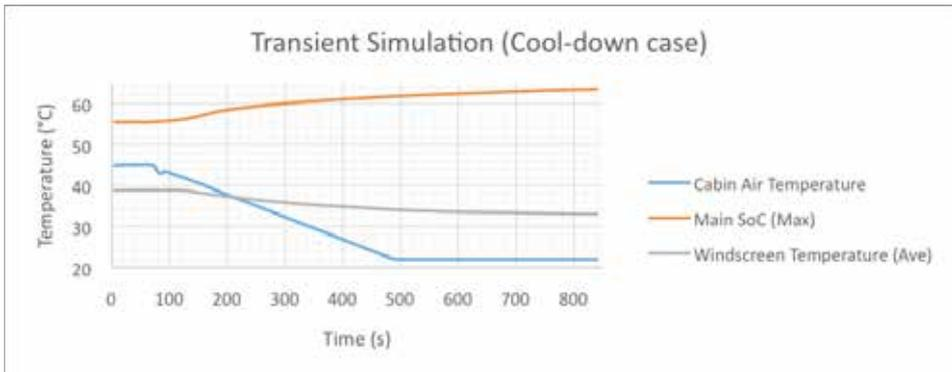
Figure 4. Key temperatures during transient cool-down simulation
