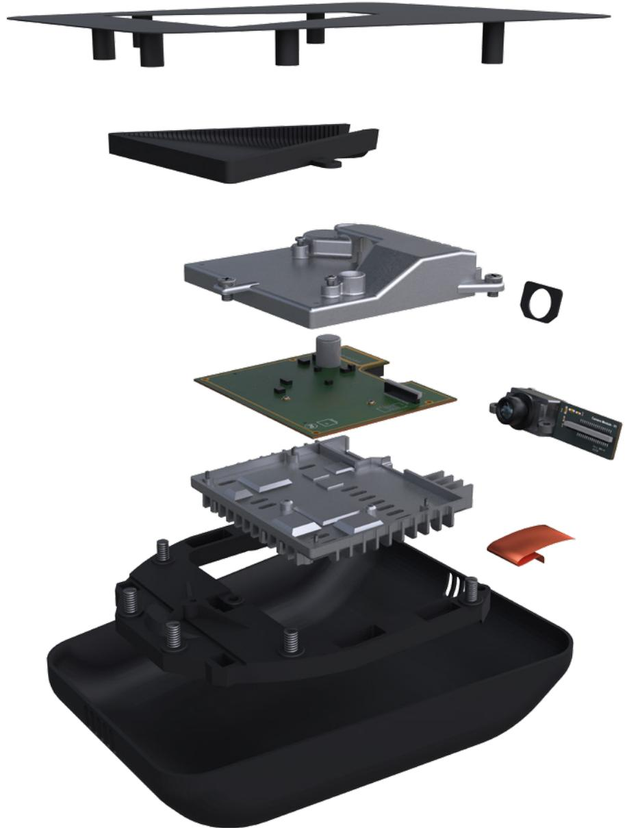
Figure 2. Exploded view of ADAS camera model
