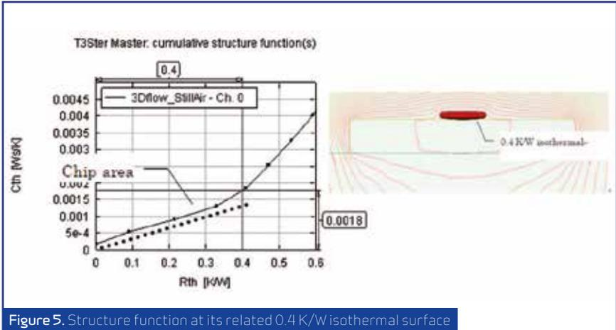
The heat source (silicon chip) is attached to a metal (copper) substrate and then attached to the FR4 board. Every material is built as a cuboid block and contact thermal resistances are not included for simplicity.
