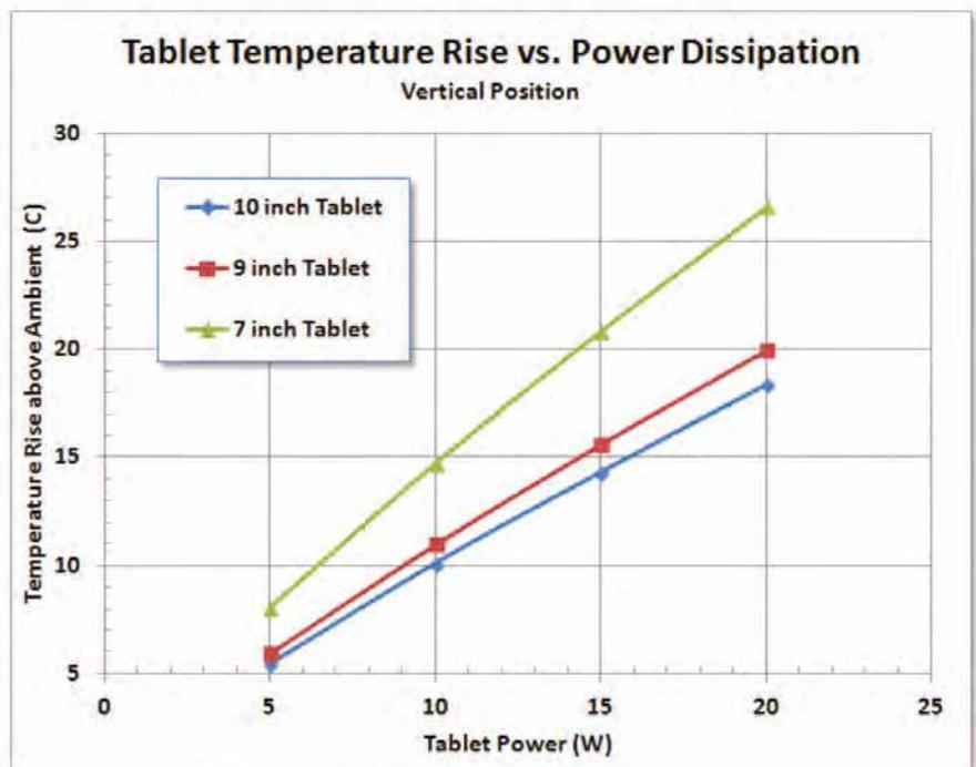
Figure 2. Temperature Rise Above Ambient as a Function of Tablet Power
