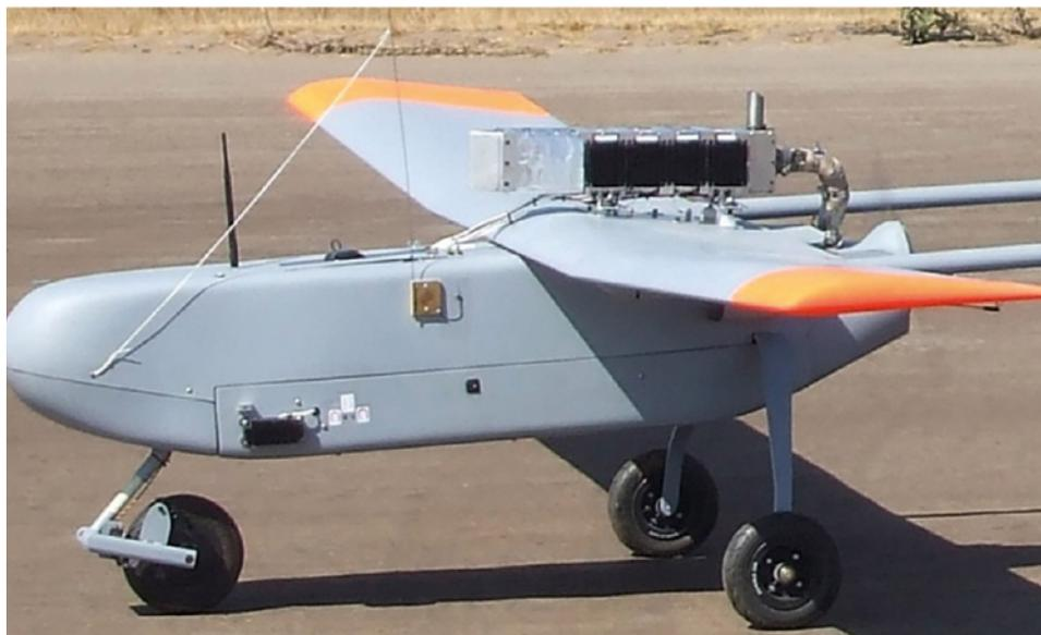
Figure 1. UAV with the EHTEG attached on top
