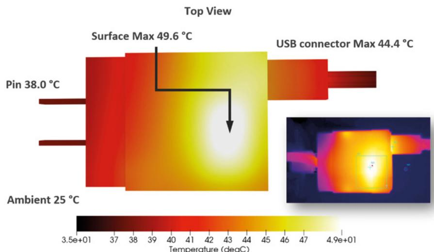
Figure 6. Final design showing surface temperature comparison with measurement
