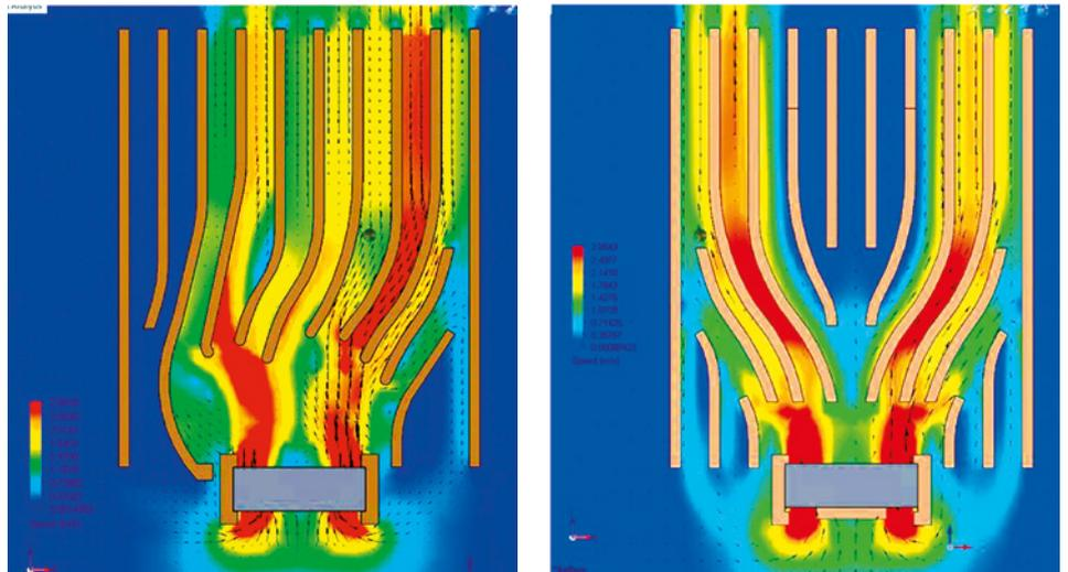
**Figure 4.** Preliminary Designs of Cast Heatsink Evaluated by Watson Marlow
