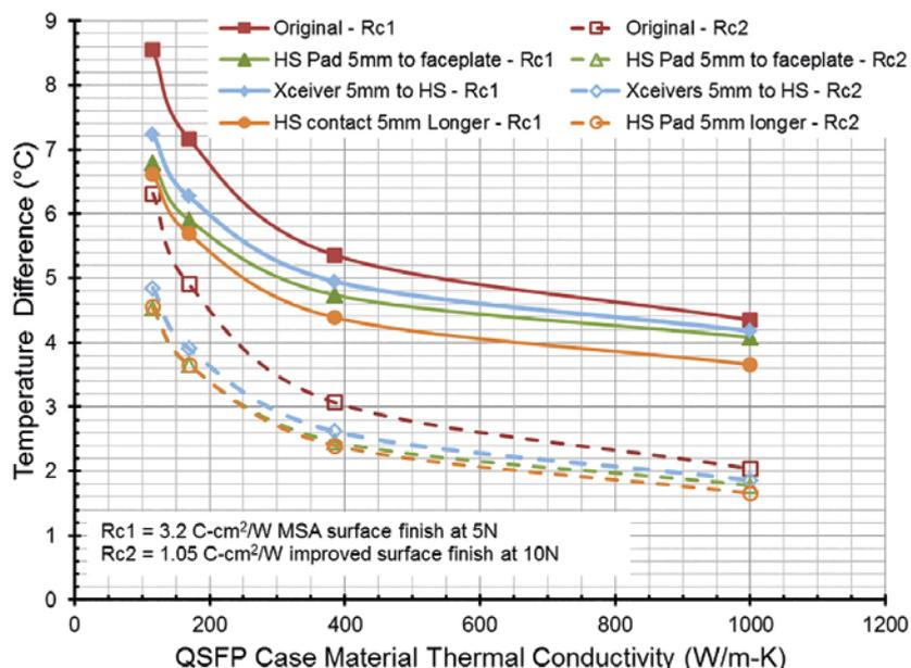
**Figure 6.** Temperature difference between QSFP hot spot monitor point and heatsink pad. Surface finishes of  $0.6 \mu\text{m Ra}$  and  $1.6 \mu\text{m Ra}$  on both heatsink and case
