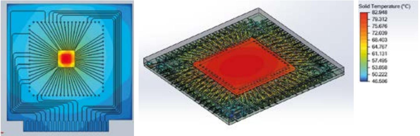
**Figure 3.** Component on JEDEC 2s2p test board in FloTHERM XT, showing internal detail including bond wires
