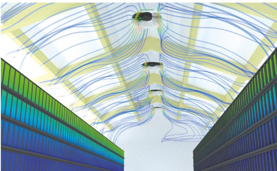
Figure 7. Typical Bitcoin Farm Ventilation Flow and Exhaust System
