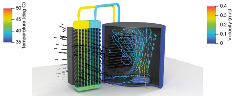
Figure 7. Design 2 Flow streamlines and cooling loop fluid temperature at 30 minutes
