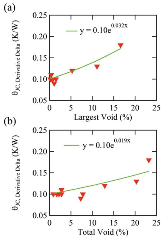
Figure 6. (a) and (b) Junction-to-case thermal resistance (for the IGBT dies) as a function of largest void as a percentage, and the total void percentage, respectively.
