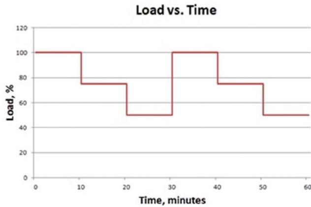
Figure 3. Power Load Profile for the ECU
