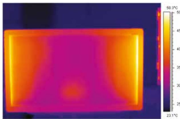
Figure 8. Infrared Picture of a Side Lit TV
