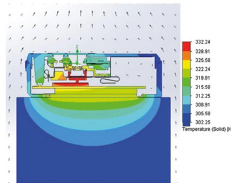
Figure 8. Beta solid temperature distribution simulation results
