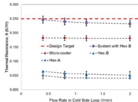
**Figure 20.** Measured thermal resistance of the heat exchangers, microcooler, and the full system assembled with compact Hex-B (a power of 175 W).
