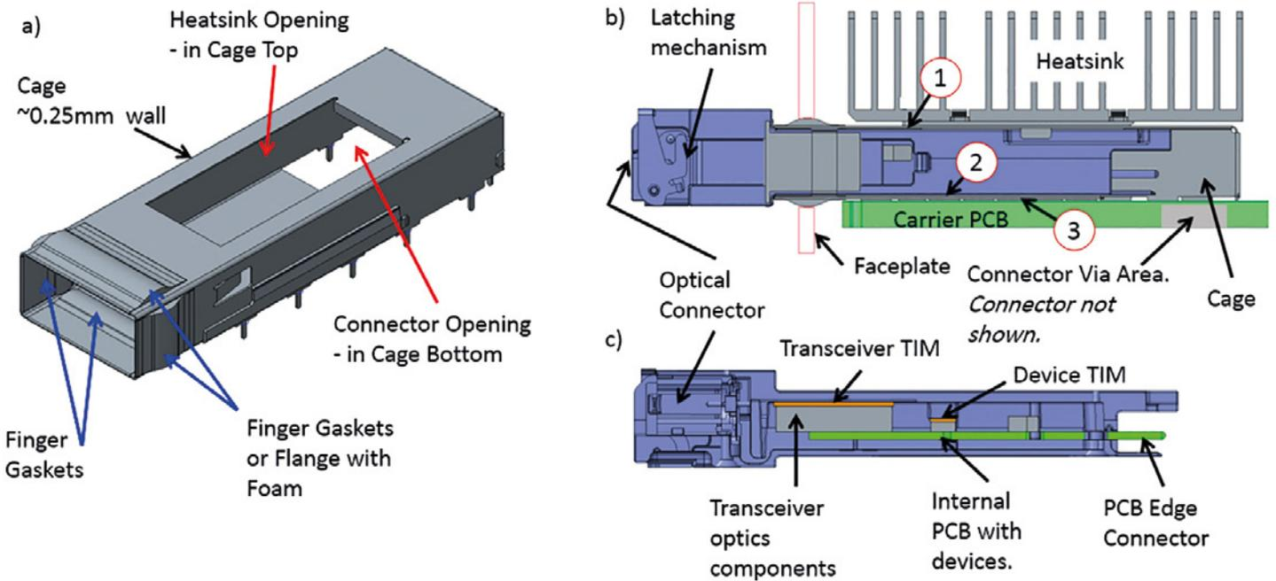
**Figure 1.** a) A typical POM cage, b) QSFP in cage section at inside edge of cage, c) QSFP section showing typical internal layout. Narrow air gap locations: 1) Module to top of cage, 2) Module to bottom of cage, 3) Bottom of cage to PCB, and not shown 4) sides of module to sides of cage.
