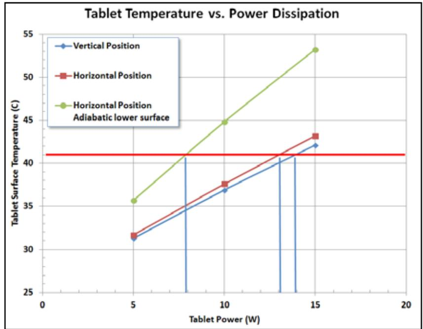
Figure 1. Total power dissipation removed by passive cooling of a tablet
