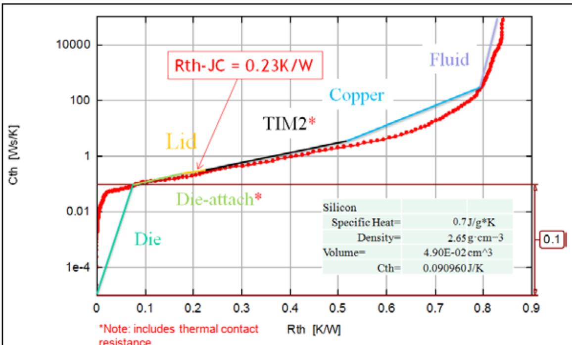
Figure 7. The cumulative structure function measured for the processor and lid using T3Ster®
