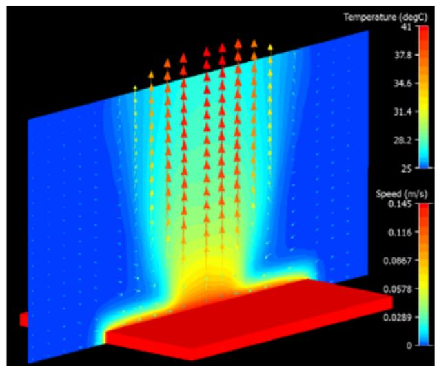
Figure 3. 41°C Isothermal tablet in horizontal position on an adiabatic surface
