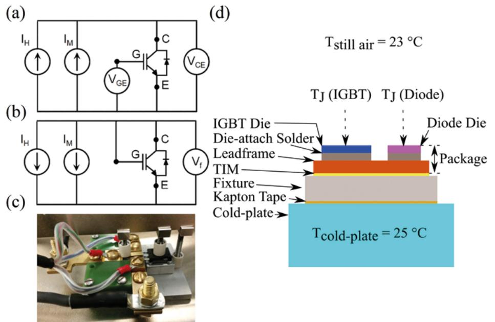
Figure 3. (a) and (b) Schematics for  $\Theta_{jC}$  (IGBT) and  $\Theta_{jC}$  (Diode) measurement, respectively. (c) Experimental setup for  $\Theta_{jC}$  (IGBT) measurement. (d) Schematic showing the cross section of different layers and boundary conditions.
