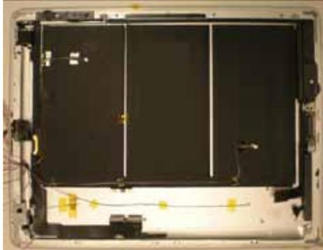
**Figure 9.** Tablet interior with thermocouples attached
