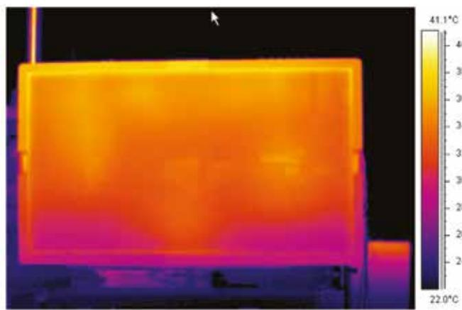
Figure 6. Infrared Picture of a Direct Lit TV
