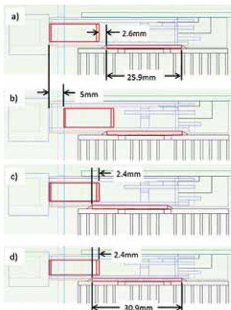
**Figure 5.** Modeling scenarios for the QSFP a) Original, b) Transceivers 5 mm closer to heatsink contact, c) Heatsink contact 5 mm closer to transceivers, d) Heatsink contact 5 mm longer towards transceivers. Transceiver location is the red rectangle on the left.
