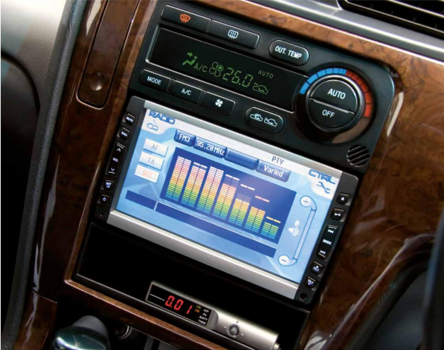
applications are highly complex systems with a large variety of mechanical and electrical components and assemblies. The design of these automotive multimedia systems has to fulfil requirements from mechanical stability and thermal management to electromagnetic compliance and optical homogeneity and therefore requires the interaction of mechanical, electrical and software engineers. Interdisciplinary knowledge is essential.
