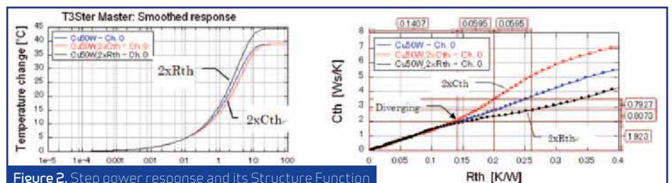
Figure 2. Step power response and its Structure Function
