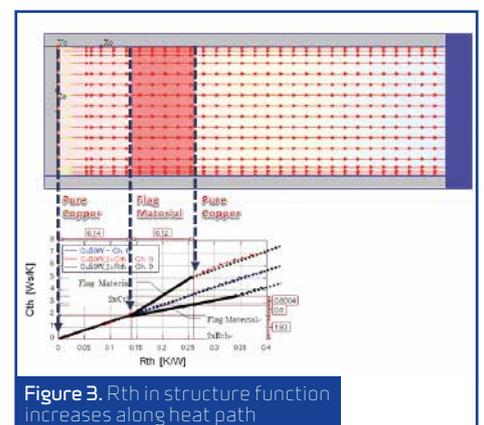
Figure 3. Rth in structure function increases along heat path
