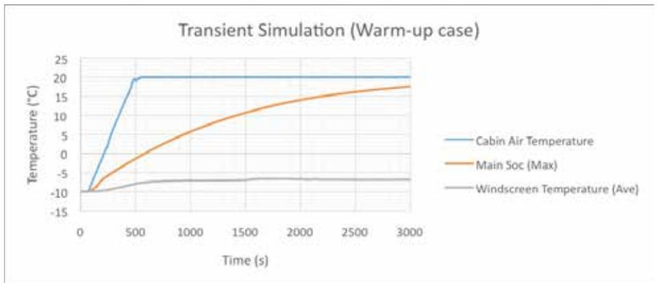
Figure 5. Key Temperatures During Transient Warm-Up Simulation
