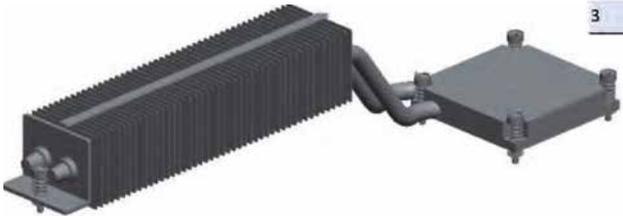
**Figure 3.** Detail of Heat Pipe Design for IC
