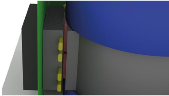
Figure 3. Design 1 cooling assembly with TEC
