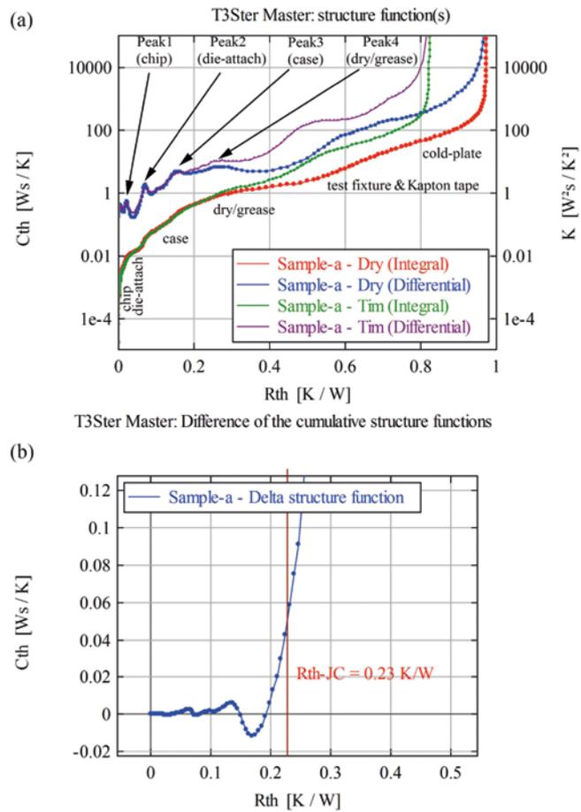
Figure 5. (a) Thermal capacitance versus thermal resistance for Sample-a showing difference in thermal paths due the change in the interface between the case of the package and
