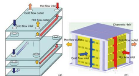
**Figure 6.** Schematic configurations of the heat exchangers investigated in this paper for (a) counter-flow configuration of commercial heat exchanger A (Hex-A) and (b) cross-flow configuration of customized heat exchanger B (Hex-B).
