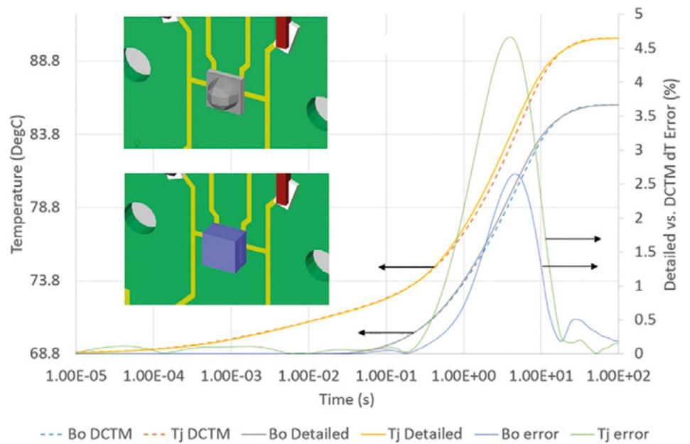
Figure 7. DCTM vs. 3D Detailed model comparisons
