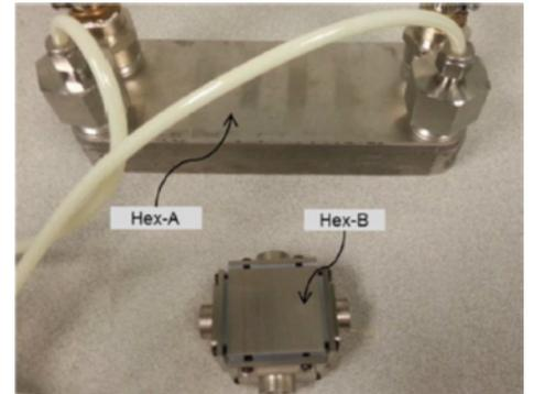
Figure 14. Comparison of the footprint size between the commercial Hex-A and the customized Hex -B
