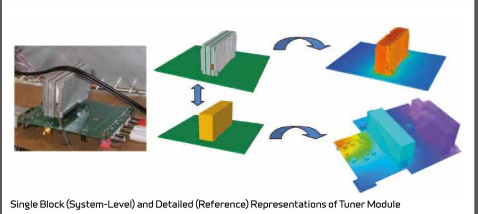
Single Block (System-Level) and Detailed (Reference) Representations of Tuner Module
