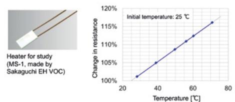
Figure 4. Ceramic heater characteristics
