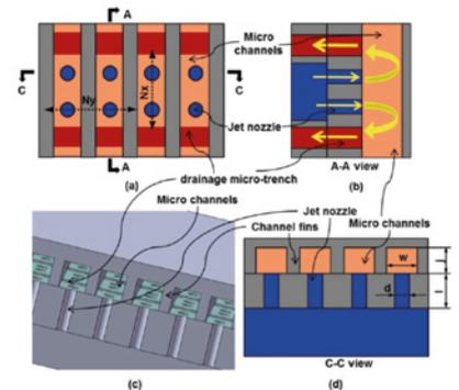
**Figure 2.** Schematic of the proposed hybrid microcooler with MDMTs design. (a) Pattern of the microchannels, jet nozzles, and MDMTs. (b) Side view of the A—A cross section. (c) 3-D isometric view. (d) C—C cross-sectional view.
