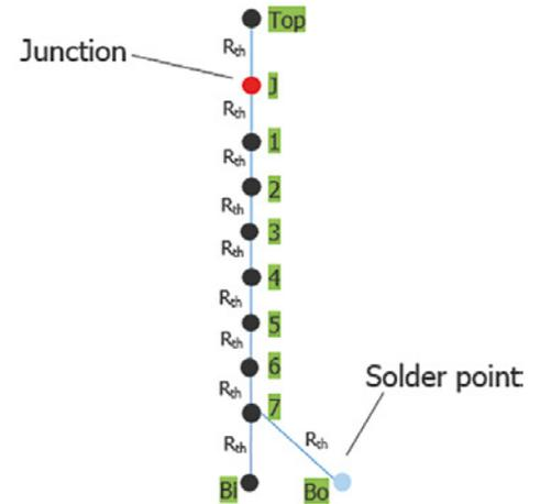
**Figure 5.** Nodal DCTM topology (thermal capacitance values at each node, not shown for clarity)
