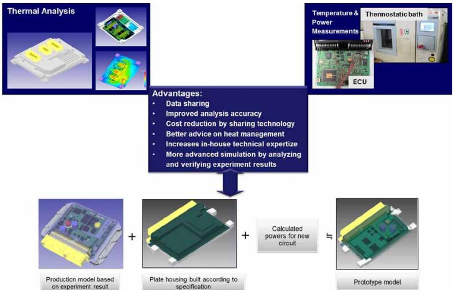
Figure 4. Advantages of centralized thermal technology - Simulation & Measurement
