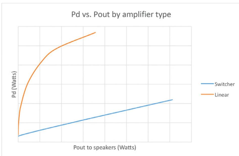
Figure 1. Power Dissipation vs. Amplifier Output Power
