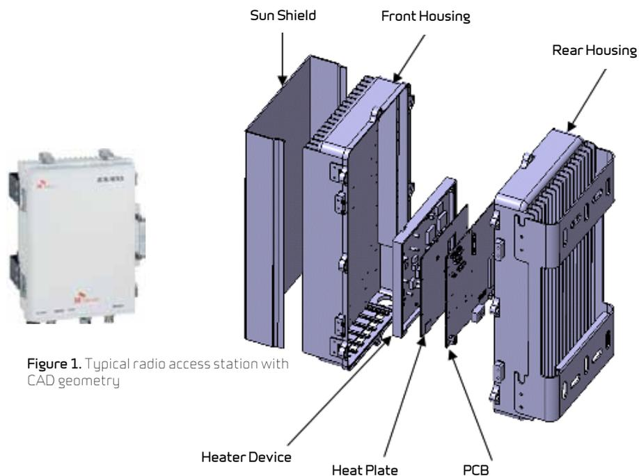
Figure 1. Typical radio access station with CAD geometry
