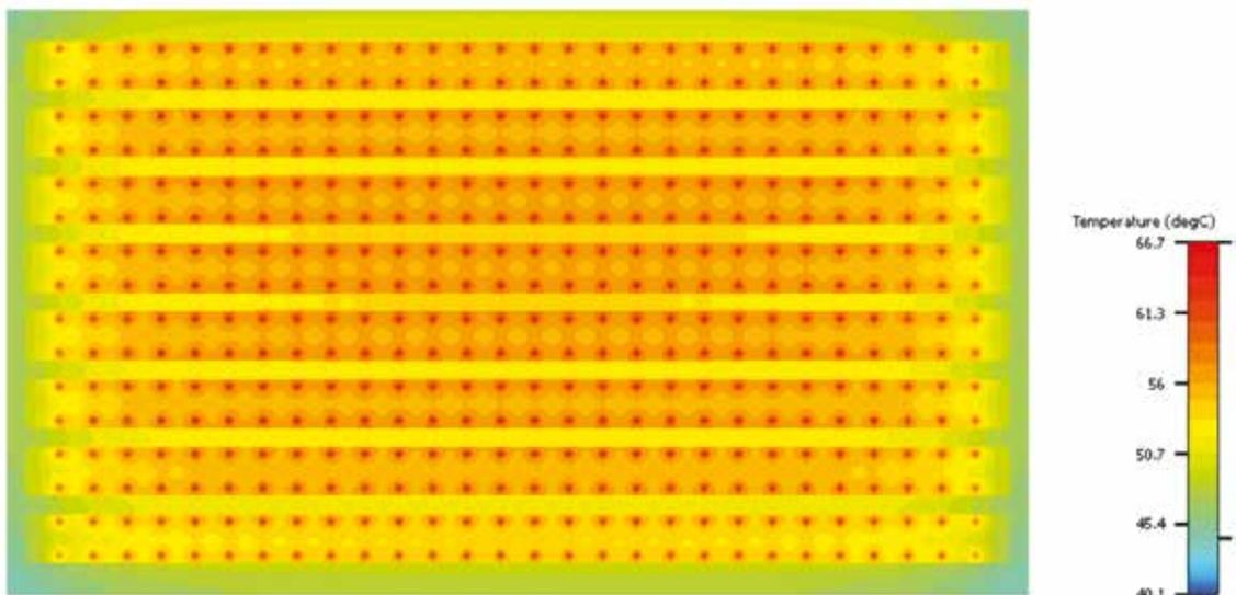
Figure 4. Calculated Temperature Distribution of the LED Boards
