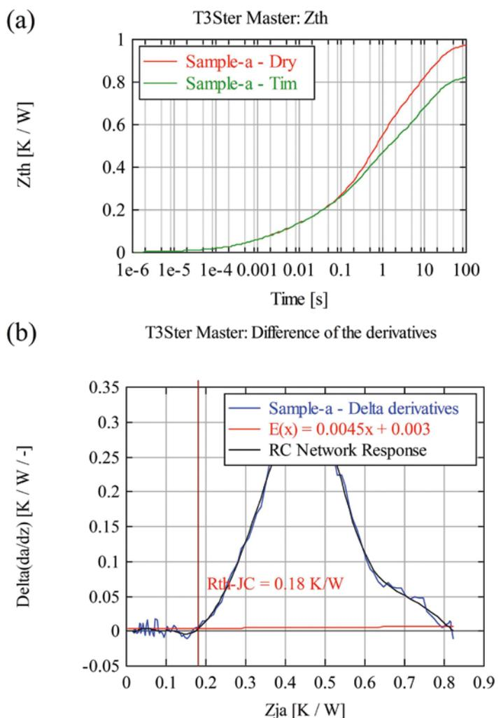
Figure 4. (a)  $Z_{th}$  curve for Sample-a measured with and without grease. (b)  $\Theta_{jC}$  evaluation following derivative delta method for Sample-a. The x value of the point of intersection between the fit curve based on RC-network response and the trend line defines  $\Theta_{jC}$ .
