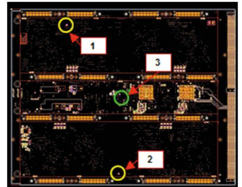
Figure 3. Mentor's logic board thermal sensors positioning
