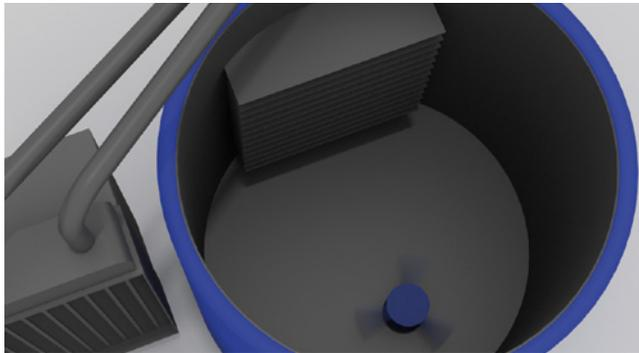
Figure 5. Design 2 internal fins with impeller
