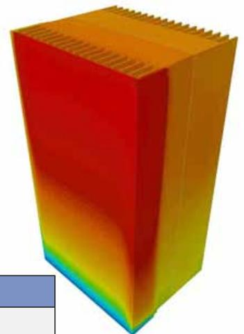
Figure 4. Boundary conditions & typical FloTHERM calculation of the base station box
