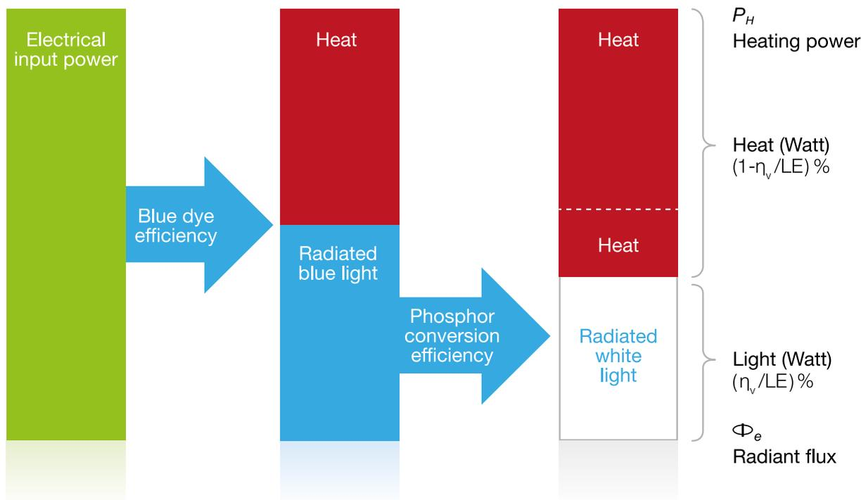
Figure 1. Power Balance of a White LED
