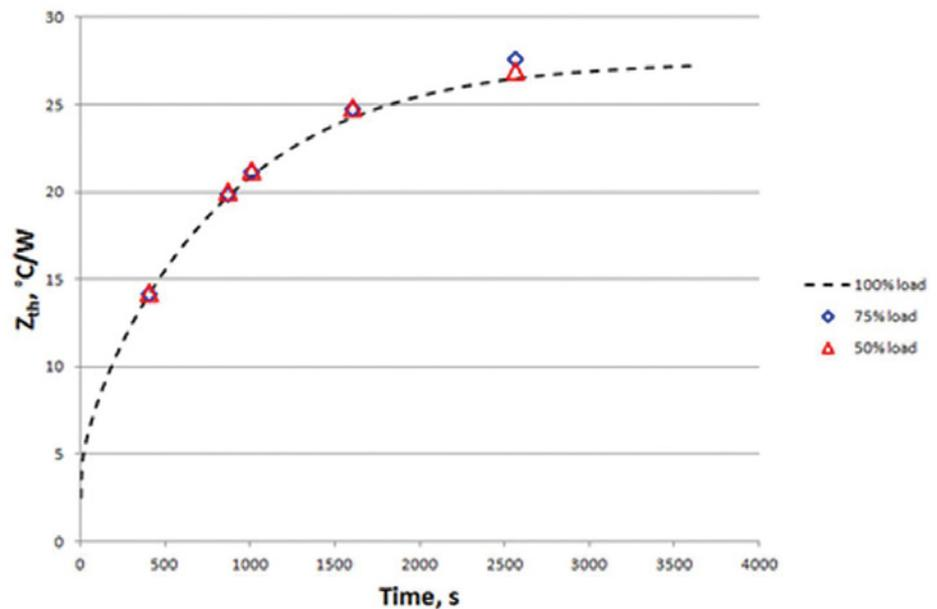
Figure 6. Comparison of dynamic thermal impedance ( $Z_{th}$ ) of 'V1907' for different loads
