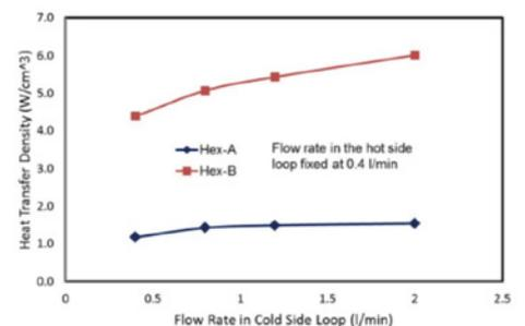
Figure 12. Comparison of heat transfer density for Hex-A and Hex-B at the specified conditions.
