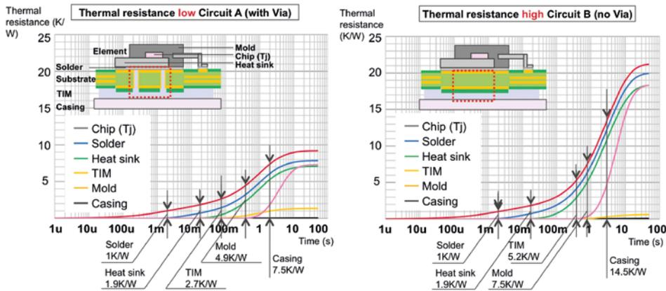
Figure 9. Temperature rise start time and thermal resistance of component for a circuit with and without a thermal via using T3Ster
