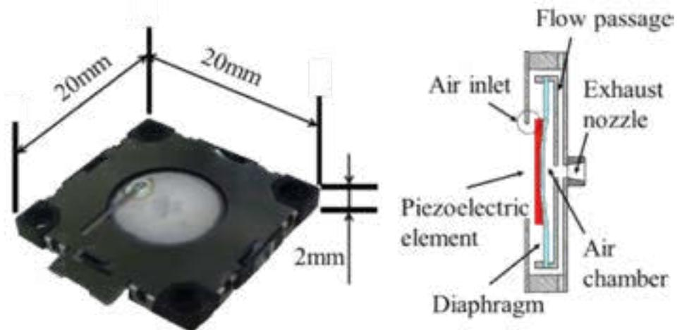
Figure 1. Murata's High-pressure Ultra-thin Microblower.
