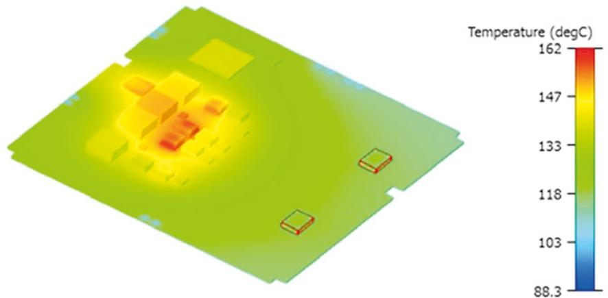
Figure 4. Temperatures of Components in Baseline model.
