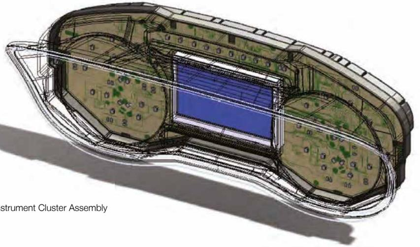
Figure 1. Instrument Cluster Assembly
