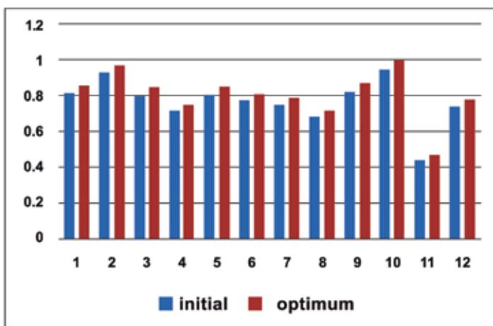
Figure 5. Difference between initial and optimal design of the base station box for the 12 key junction temperatures
