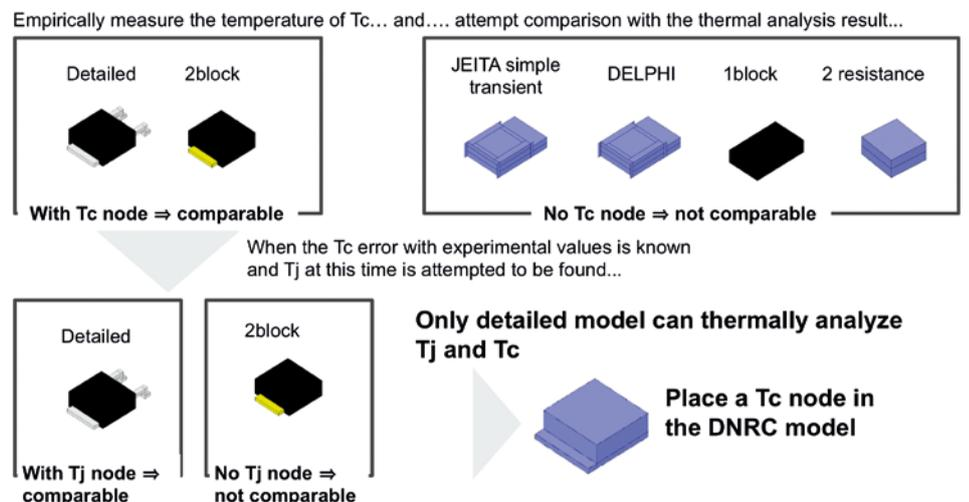
Figure 14. Innovation 1 - Temperature of the part for coupling with CFD analysis is known
