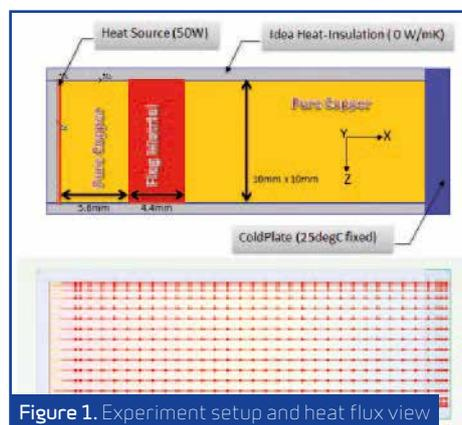
Figure 1. Experiment setup and heat flux view.
