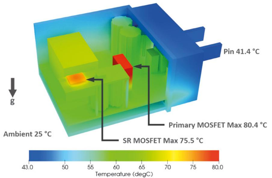
Figure 4. Initial design showing internal hot spots
