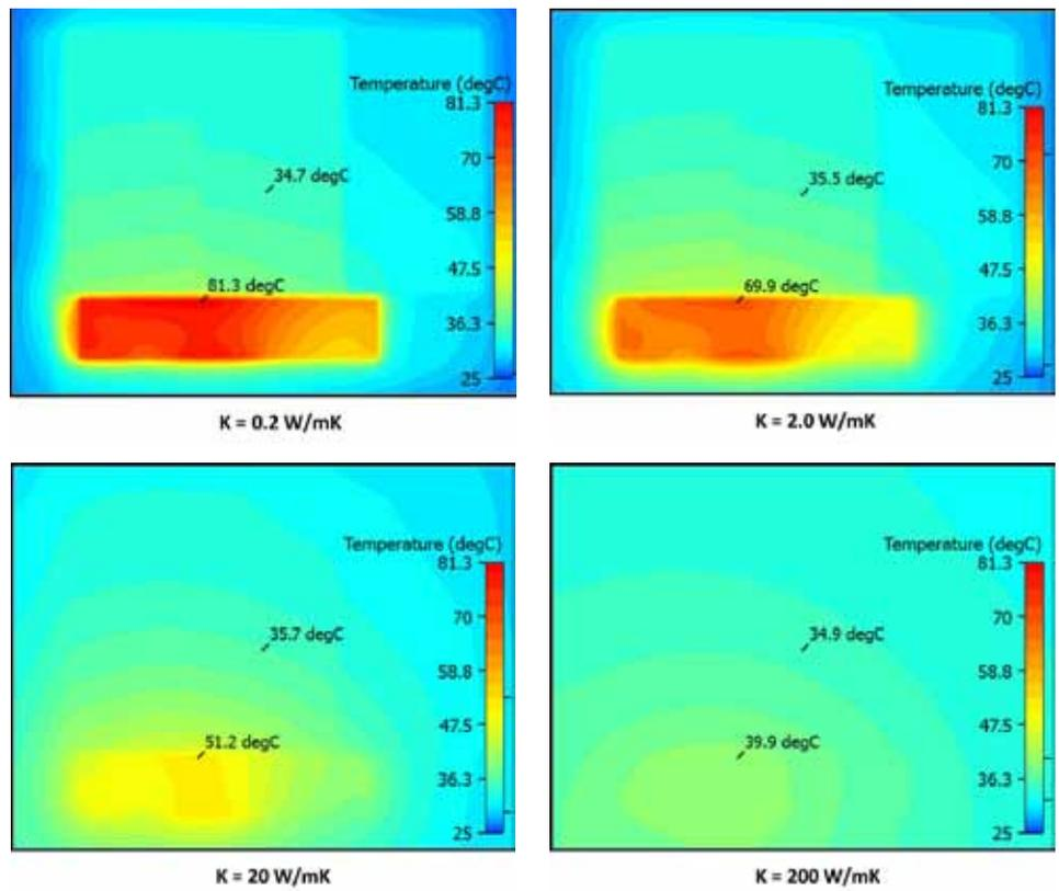
Figure 5. Back-side hot spot temperature change as a function of case thermal conductivity
