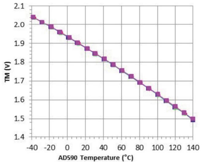
**Figure 9.** Temperature monitor (TM) volts versus sensor temperature.
