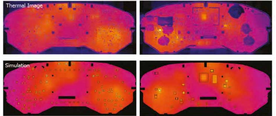
the cluster full assembly to determine its performance in worst case conditions at an air ambient temperature of 85°C.
