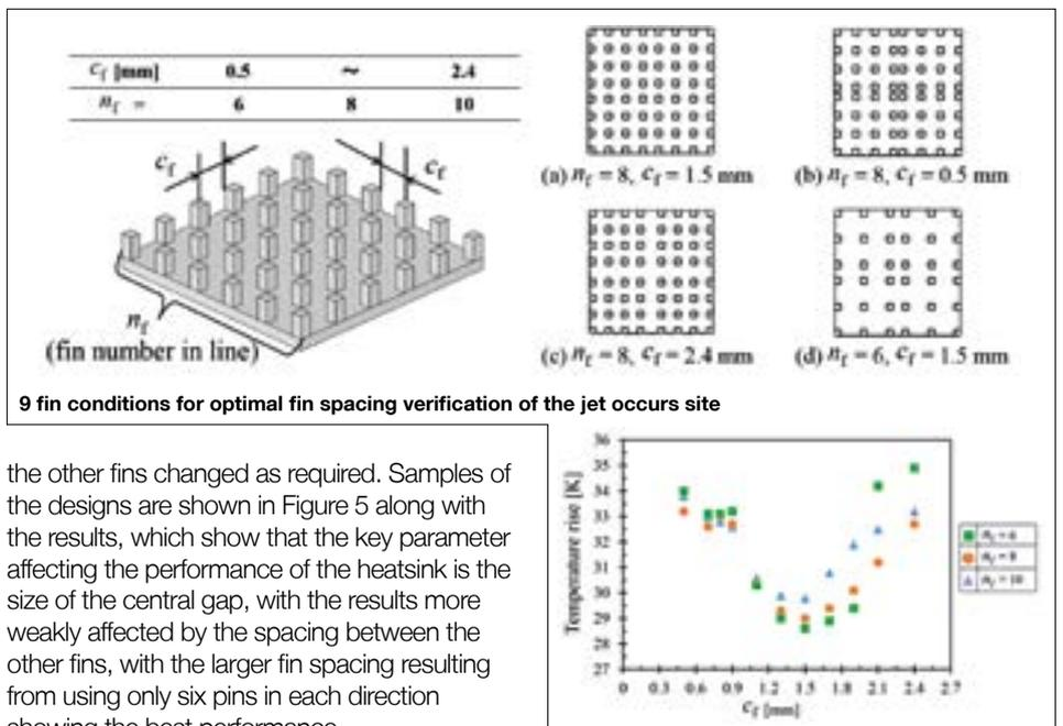
the other fins changed as required. Samples of the designs are shown in Figure 5 along with the results, which show that the key parameter affecting the performance of the heatsink is the size of the central gap, with the results more weakly affected by the spacing between the other fins, with the larger fin spacing resulting from using only six pins in each direction showing the best performance.
