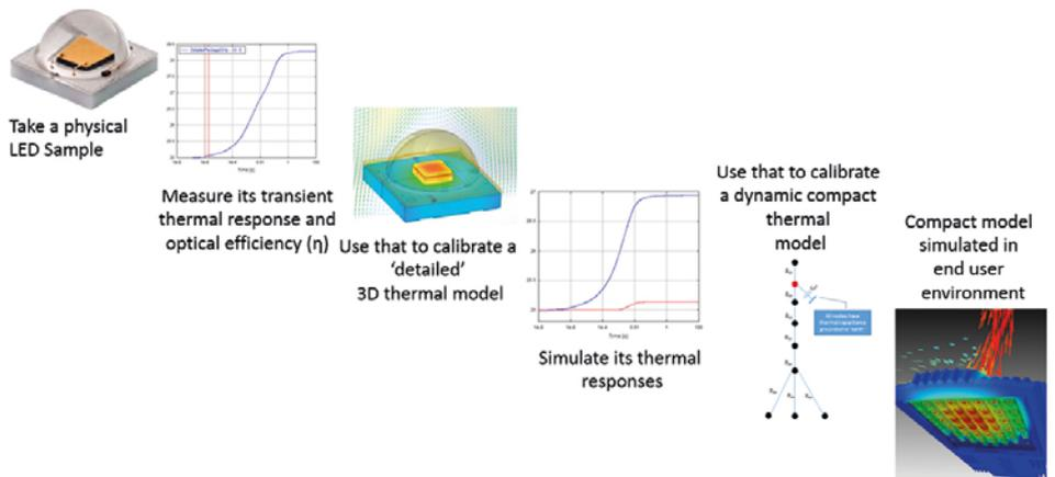
Figure 2. Dynamic compact thermal model extraction process
