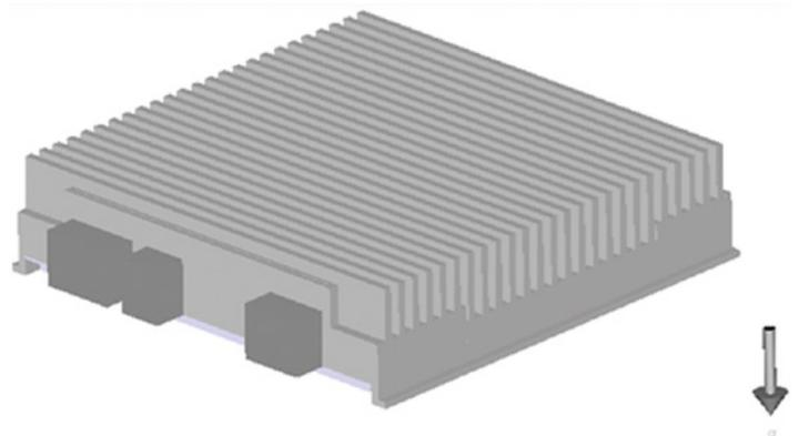
Figure 2. FloTHERM Model of ECU showing Finned Housing
