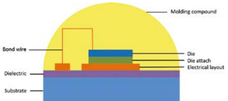
Figure 1. Structure of a high power LED-package
