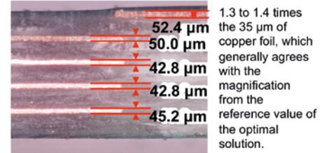
Figure 12. Validation of optimal solution with a structural survey of real substrate samples
