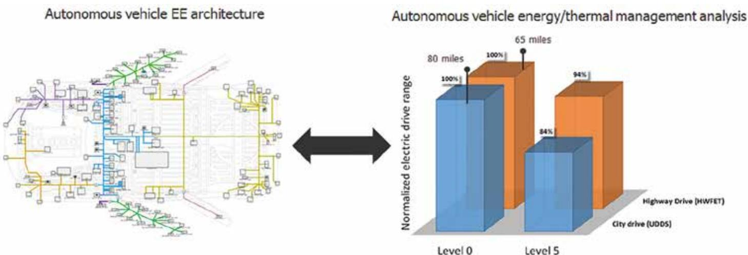
**Figure 3.** Impact of Level 5 autonomous vehicle system integration on electric drive range. In this example, Level 5 autonomous electric vehicle (80 miles electric range with 80kW front motor drive unit) is simulated where vehicle EE architecture (simulated using Mentor's Captial software) includes 30 sensors, DRS360 centralized sensor fusion and ECUs for steering and braking. Electric drive range is simulated at 25°C ambient conditions using FloMASTER based e-powertrain simulation framework.
