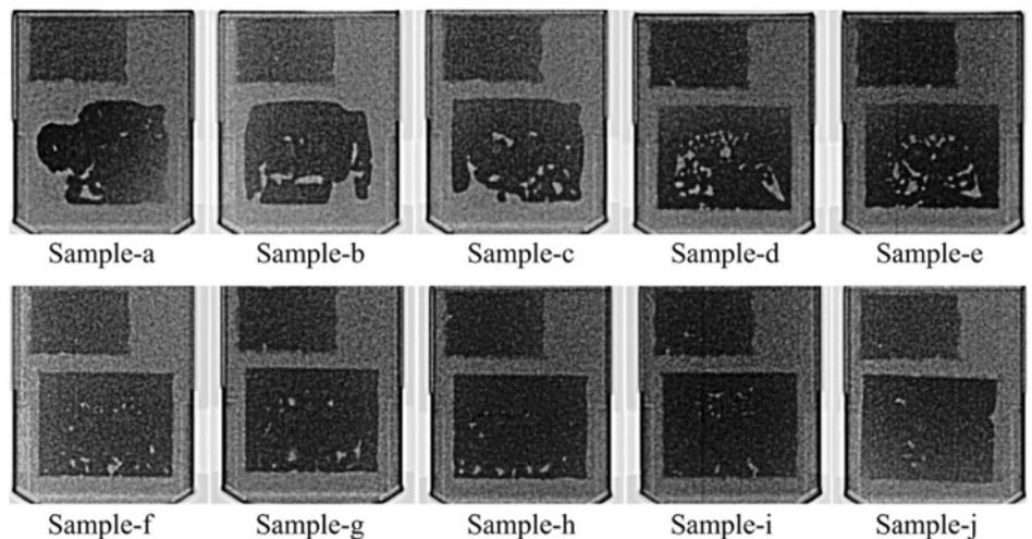
Figure 1. Samples in decreasing order of die-attach voiding under IGBT die
