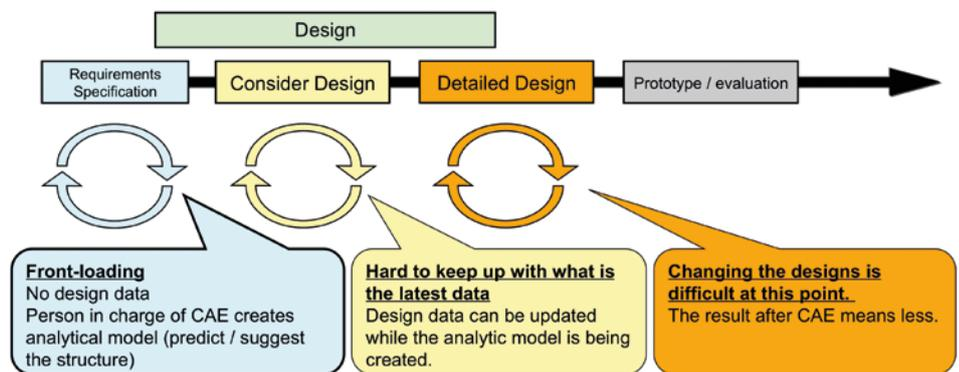
Figure 1. Fujifilm Camera Design Process
