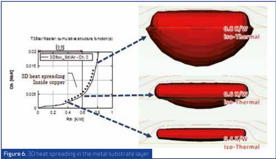
Figure 6. 3D heat spreading in the metal substrate layer
