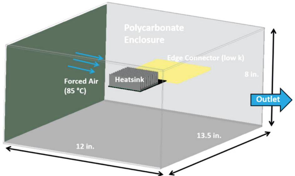
Figure 6. Package with heatsink in a forced-air environment
