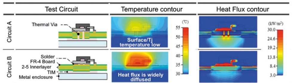
The calculation of element Tj depends on the thermal resistance of the substrate
