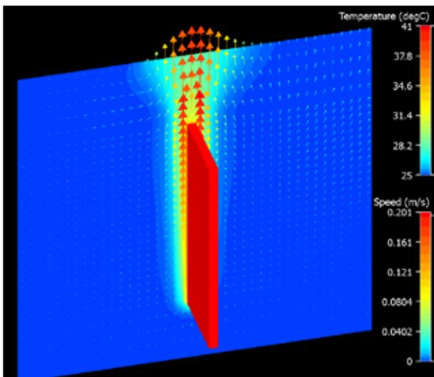
Figure 2. 41°C Isothermal tablet in vertical position
