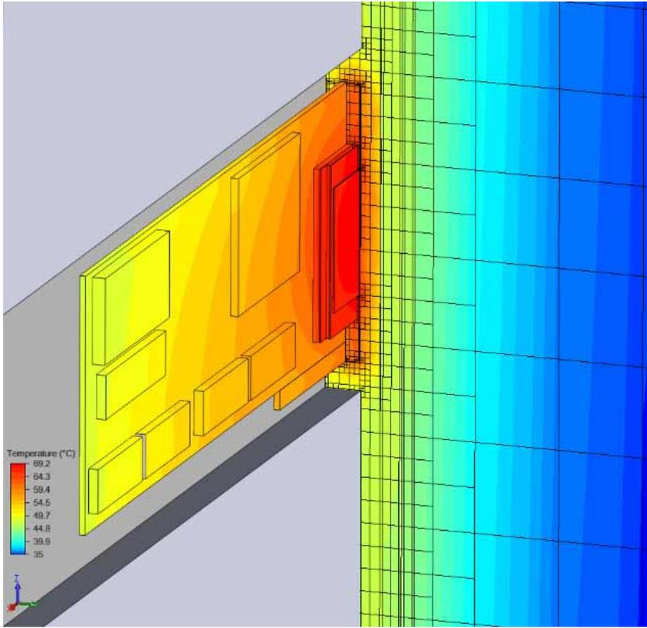
Figure 4. Detailed model of the PCB created in FloTHERM®XT
