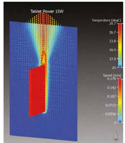
Figure 1. FloTHERM® CFD Model of a 10 Inch Tablet in a Vertical Orientation
