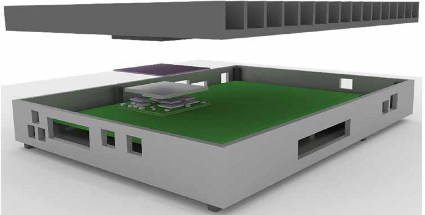
**Figure 1.** Rendering of a reference solution for an IoT module
