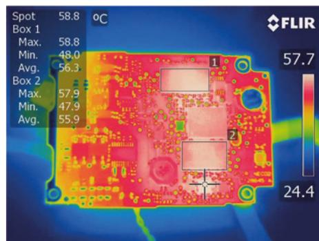
Figure 4. Alpha phase PCB top surface IR image
