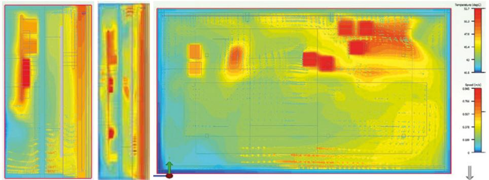
Figure 2. Typical results with flow, total dissipation 18.5W
