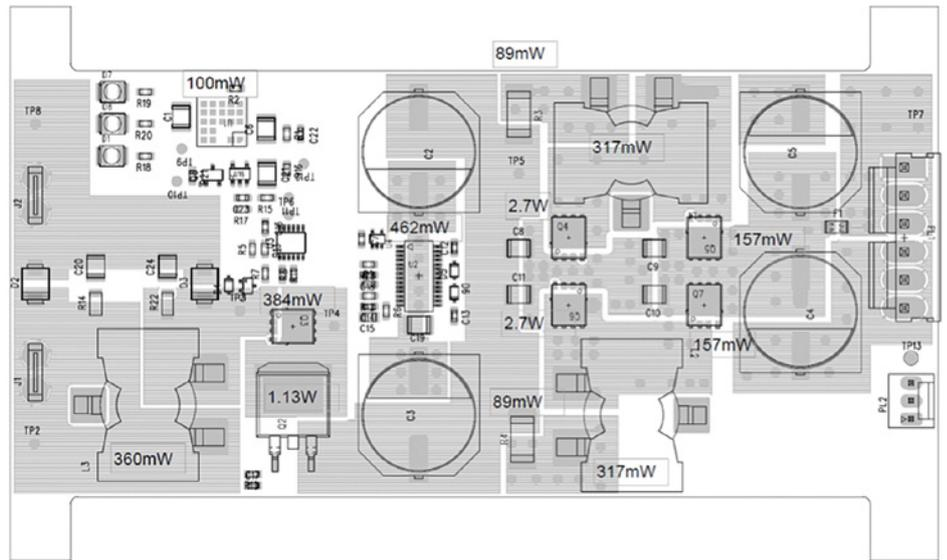
**Figure 3.** PCB component layout drawing from PADS
