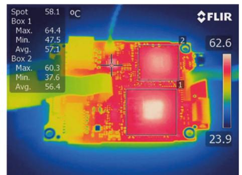
Figure 5. Alpha phase PCB bottom surface IR image
