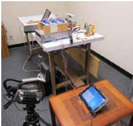
Figure 8. Lab setup with IR camera, power measurement and temperature logging equipment
