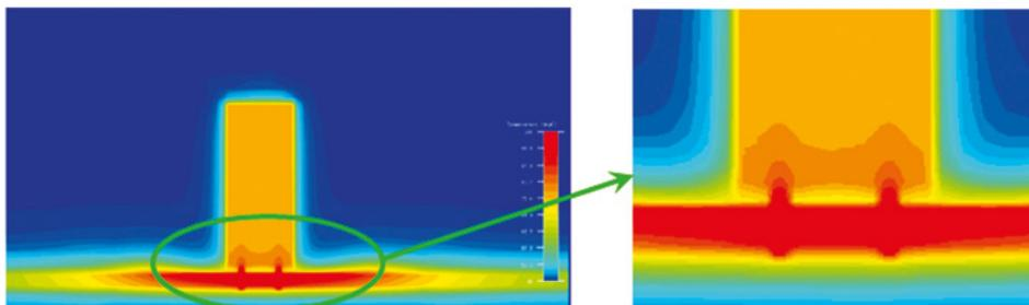
**Figure 10.** Capacitor temperature field in the FloTHERM simulation
