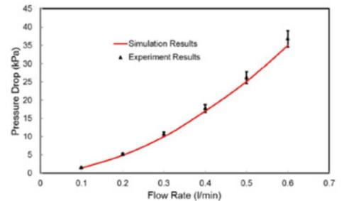
Figure 16. Pressure drop in Microcooler
